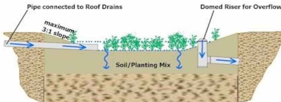
Figure B-5: Typical Rain Garden/Bioretention Area
